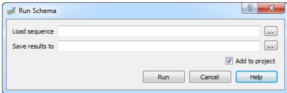
Select the *Sequence* to analyze with the schema and browse for the file in GenBank format to *Save results to*. Optionally, check the *Add to project* button to add the created result file to the active project. Press the *Run* button.
