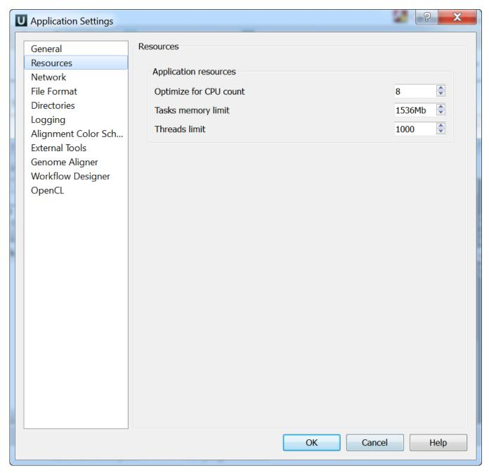
On the Resources tab you can set resources that can be used by the application: Optimize for CPU count, Tasks memory limit and Threads limit.
